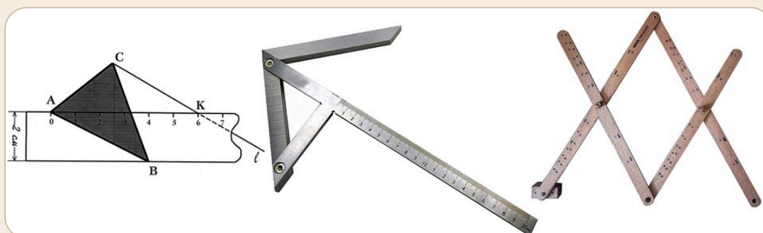
Bibikov's agrometer, a diameter gauge and centre finder (centring square), and a pantograph · Source
