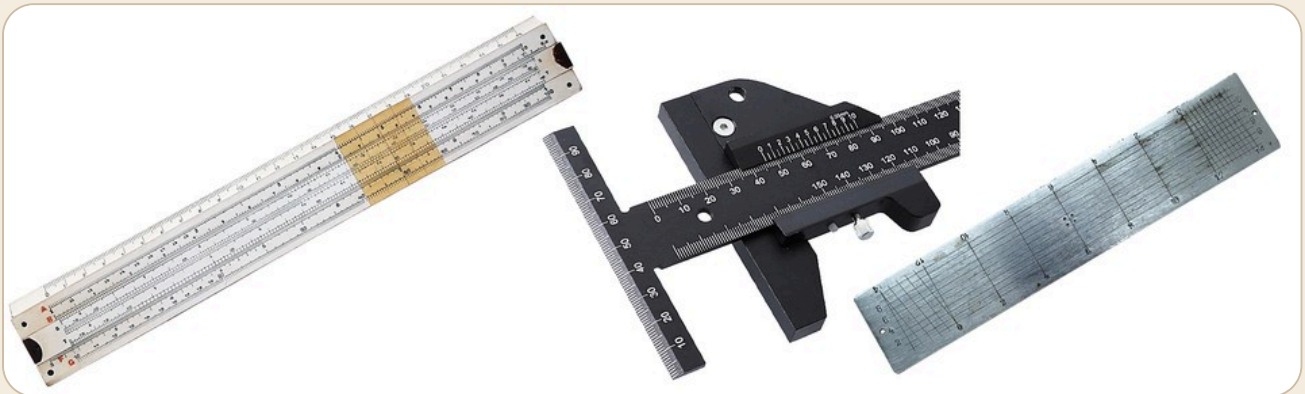
A slide rule, a ruler with a vernier scale and a ruler with a diagonal scale · Source
