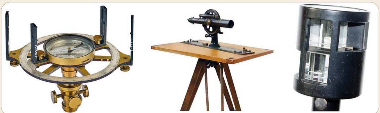
A surveying astrolabe, a plane table and a surveyor’s cross with two pentaprisms · Source
