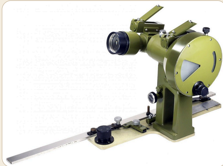
Shiryayev KVSh-8 height-measuring alidade (1970) · Source
