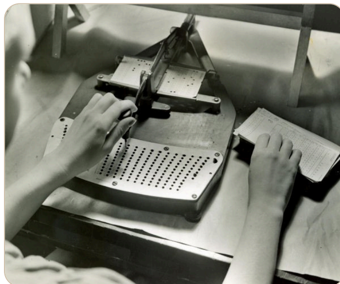
A pantograph punch used to create punched cards in Hollerith's system · Source
