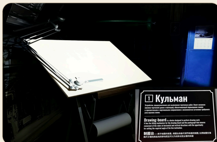
A drafting machine: an improved drawing board · Source
