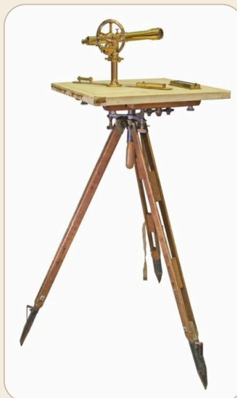
Plane-table set: tripod and plane table (first half of the 20th century), drawing board (1950s) and telescopic alidade. From the Open Collection of the Museum of History and Labour Glory of the Zavolzhye Motor Plant (ZMZ) · Source
